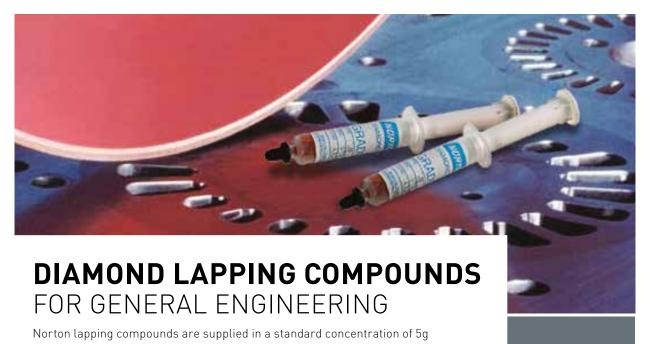
dispenser syringes. Perfectly sized synthetic diamond powder is mixed with a paste. When used, this compound should be diluted with water or alcohol.
