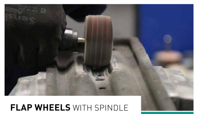
Flap wheels conform to intricate shapes and contours. Designed to deliver a consistent finish with a uniform rate of cut, they wear away evenly and without residue, continually exposing fresh abrasives.
