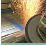
STEP 4 **WELD SEAM REMOVAL**
