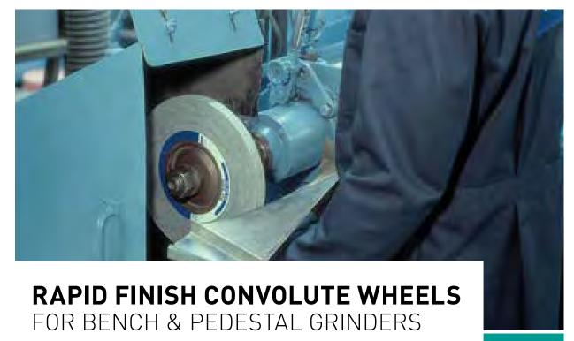
Convolute wheels are formed by wrapping non-woven web material around a centre core and bonding the layers together to create an abrasive wheel. Wheels are available in different diameters, grades and densities for burr, flash and rust removal, reducing surface roughness, blending welds and scratch patterns on stainless steel, polishing welds and applying decorative finishes.
