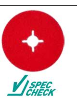
Grinding on stainless generates a considerable amount of heat; always use a Norton Quantum disc with 'supersize' layer, a grinding aid added to the disc to reduce heat generation and improve cut and finish quality. Typically, a coarse grit disc is used when grinding MIG welds and a finer grit disc is used when grinding TIG welds.
