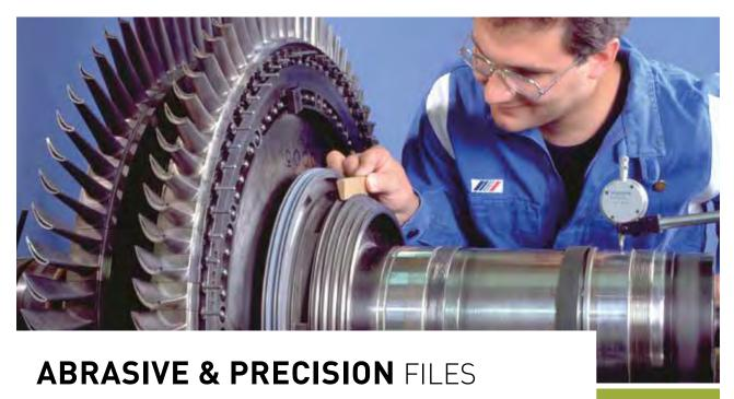
Norton abrasive files hold their shape while imparting the finest, most uniform finish on precision machine parts, and in tool and die making.
