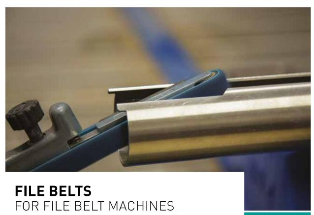
Norton provides a wide range of file belts tailored for exceptional performance on complex shapes and contours. Portable file belt sanders have replaced tedious hand filing and sanding. They were first introduced in pneumatic form and are now also available in electric form. The belts listed are popular stock sizes, but additional sizes, specifications, backing materials, and edge scallops are available made-to-order.
