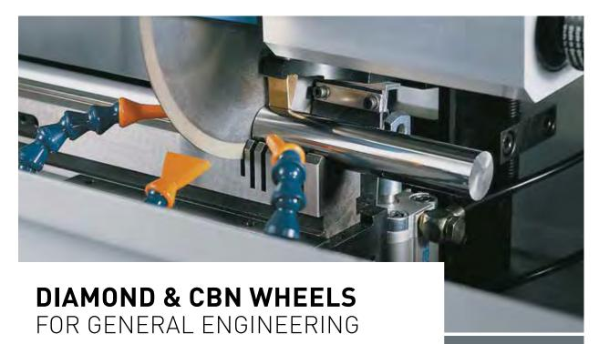
Norton offers a small assortment of standard resin-bonded cut-off grinding wheels. The specified diamond cut-off wheels cut hard, short-chipping and wear-resistant materials such as glass, ceramics and carbide. The contained CBN cut-off wheels are ideal for machining high-speed steel, hardened steel, 55 HRC and magnetic materials.
